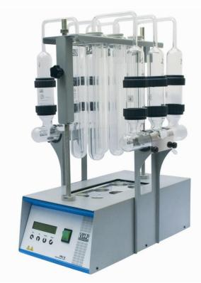
In the large majority of food and feed products the fats contained are chemically bonded with other components. For the determination of the total fat content of these samples, preliminary hydrolysis using hydrochloric acid followed by filtration and washing, is indispensible in order to free the fat molecules ready for extraction.
